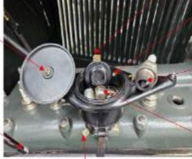
Place a couple of drops of oil in the oiler for the lower shaft bushing.
